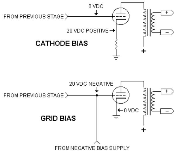
**Fig 5** Methods of biasing a tube amplifier stage
